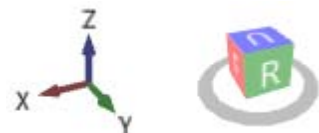
Fig. 174: Auxiliary objects from the 3D scene ( Left – coordinate system; Right – view cube).
