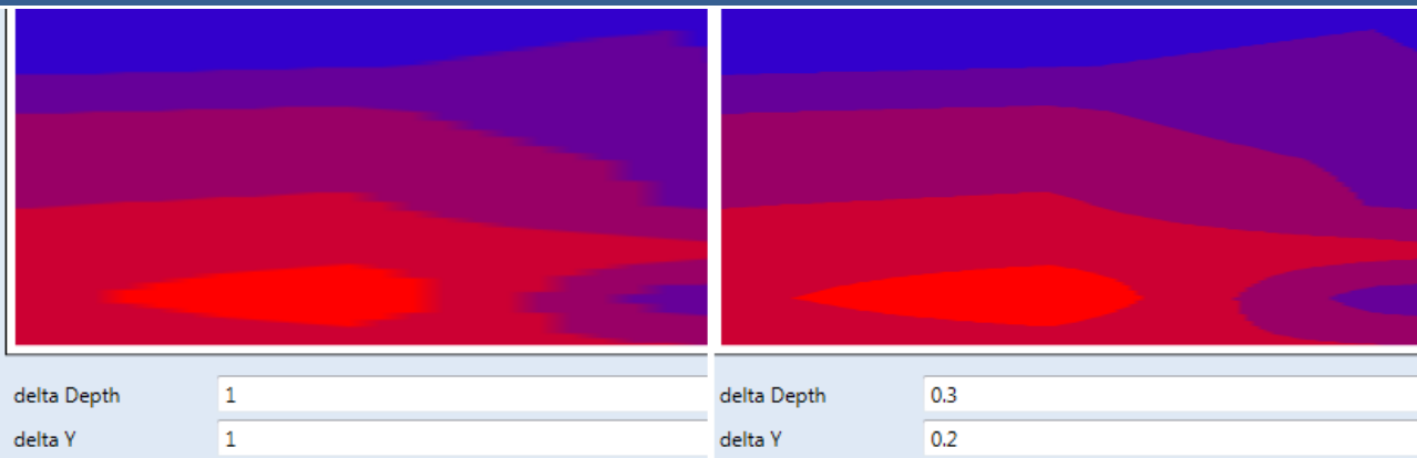
Fig. 53: Two examples of heat map resolution settings ( Left – predefined resolution; Right – modified resolution).
