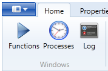
Fig. 58: The position of the “ Application.Functions, Application.Processes and Application.Log ” commands in the ribbon toolbar.
